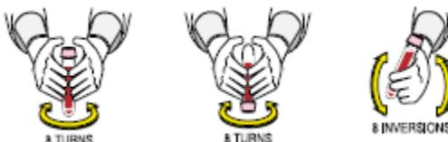
3. Repeat steps 2a to 2c three times. Visually inspect the tube contents for complete re-suspension. If necessary, repeat steps 2a to 2c until tube contents are uniformly suspended.
